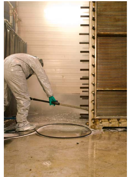
Removing the side panels on a Compabloc gives full access to all channels for cleaning
