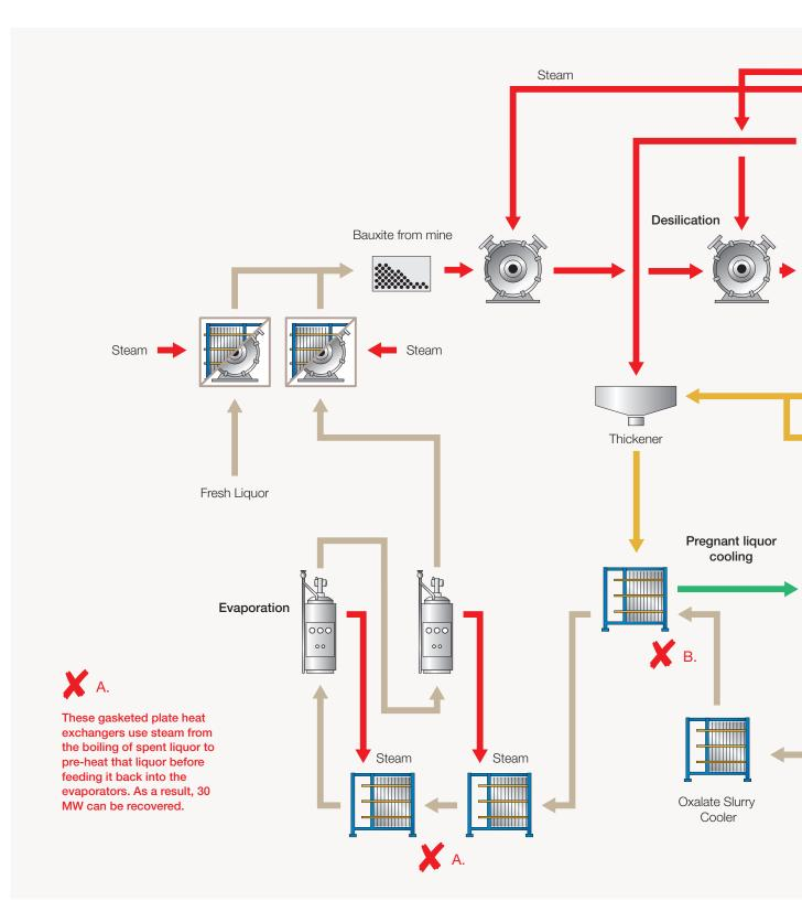
In alumina production, digestion, evaporation, liquor heating and other energy-intensive extraction processes can be tapped for vast amounts of heat. Heat that can be fed right back into the flow, with an unparalleled yield.
