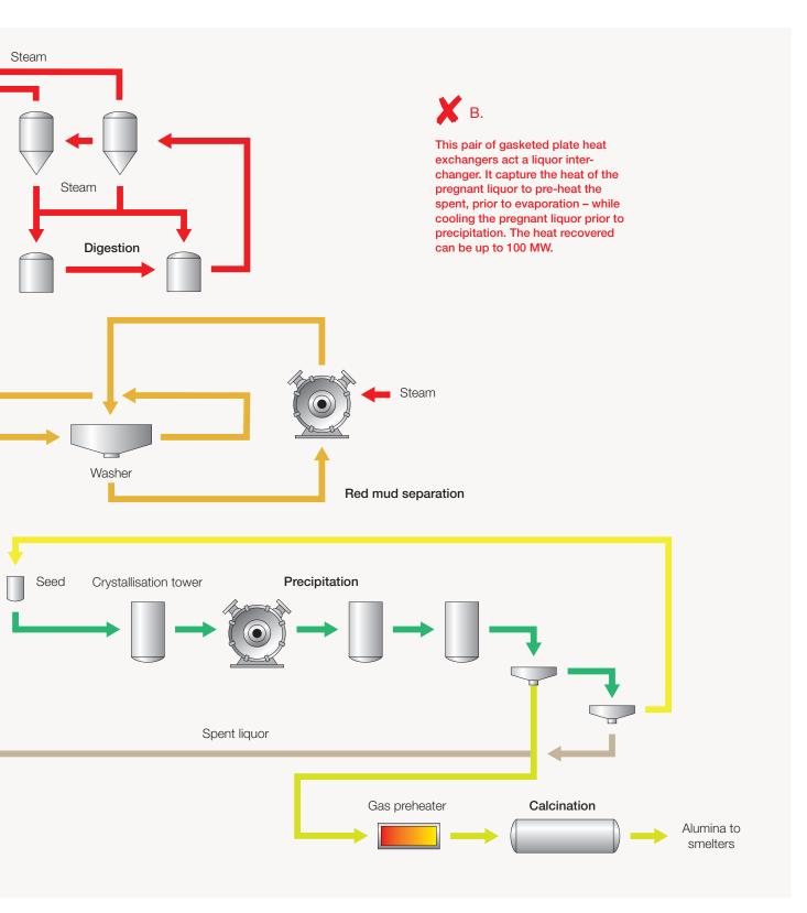
turbulence and large heat-transfer areas combine to squeeze up to 30% more energy out of every heat flow than conventional shell-and-tube units.
